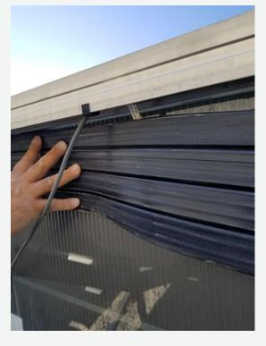
In order to couple the panel to the recyclable flexible elastomer device and not shock the panel or break the glass, Enertopia has developed a breakthrough technology that acts like a thermal check valve allowing heat to go one way, away from the back of the panel
